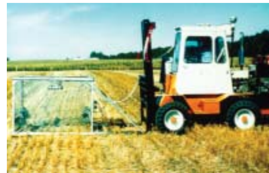
The gas collection chamber is measuring carbon dioxide emissions on undisturbed (no till) soil after winter wheat harvest.
