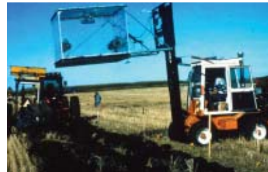
A gas collection chamber, designed by ARS scientists in MN, is used to capture carbon dioxide emissions from the soil after different management systems. This view shows it being lowered to the soil surface immediately after moldboard plowing winter wheat stubble.
